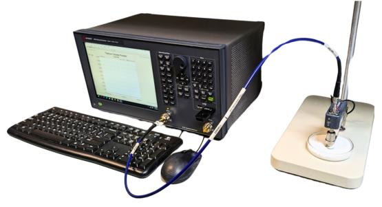
Dielectric property data is necessary to determine the power requirements and performance of industrial microware systems.
