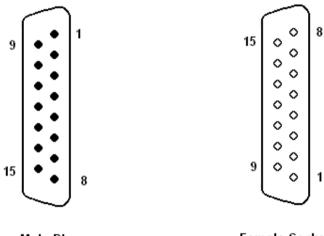
Male Plug (Front View) Amplifier Connector Female Socket (Front View) Matching Interface
