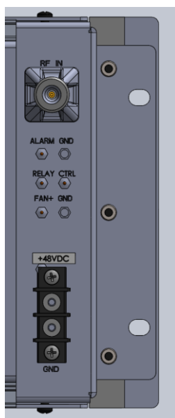
Figure 2-2. C5 Series Amplifier, Rear View Right
